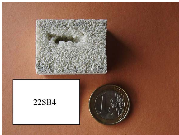
Fig. 1. Cross-section of 22SB4 cordierite foam impregnated in a slurry containing 65 wt.% solid load.
